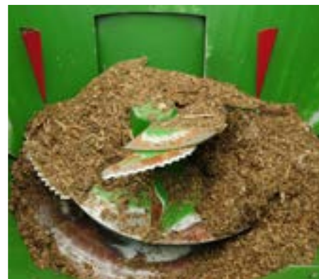
Auger with optimal shape increases efficiency of mixing
