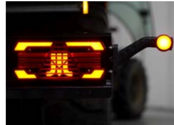
Installation of 12V LED lighting with marker lights
