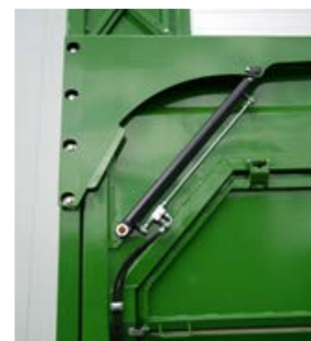
Hydraulic system of the tailgate with rubber sealing gasket
