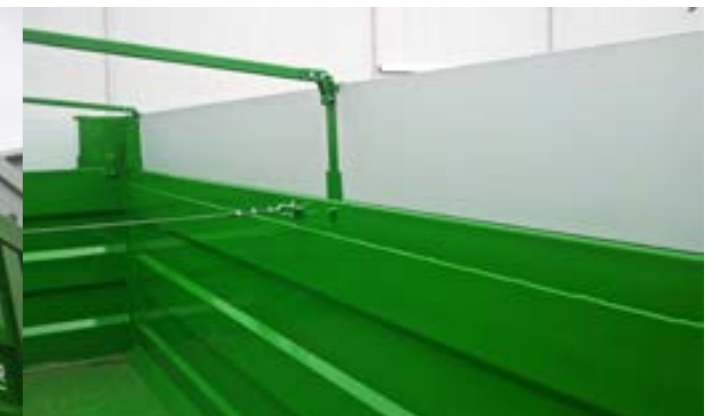
1500 mm | 4'11" ft walls + 400 mm | 14" ft aluminum extensions
