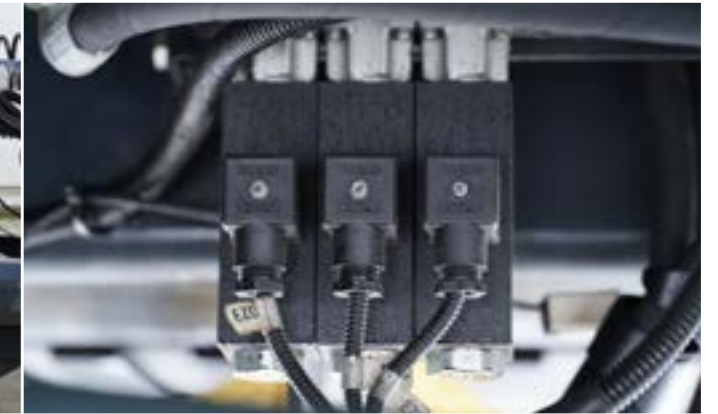
Central hydraulic system with distributor
