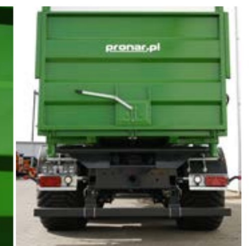
Grain chute with locking mechanism
